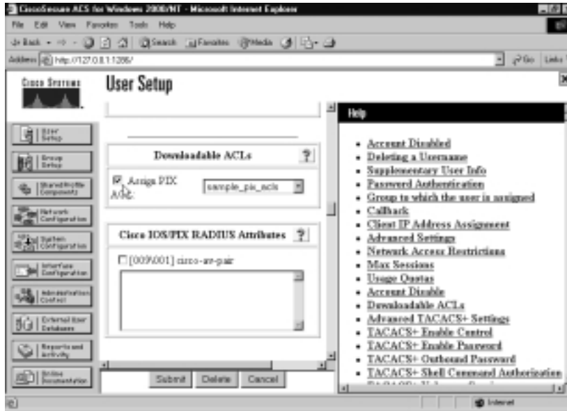
Figure 5.45 Cisco Secure ACS: Assigning Downloadable ACL
