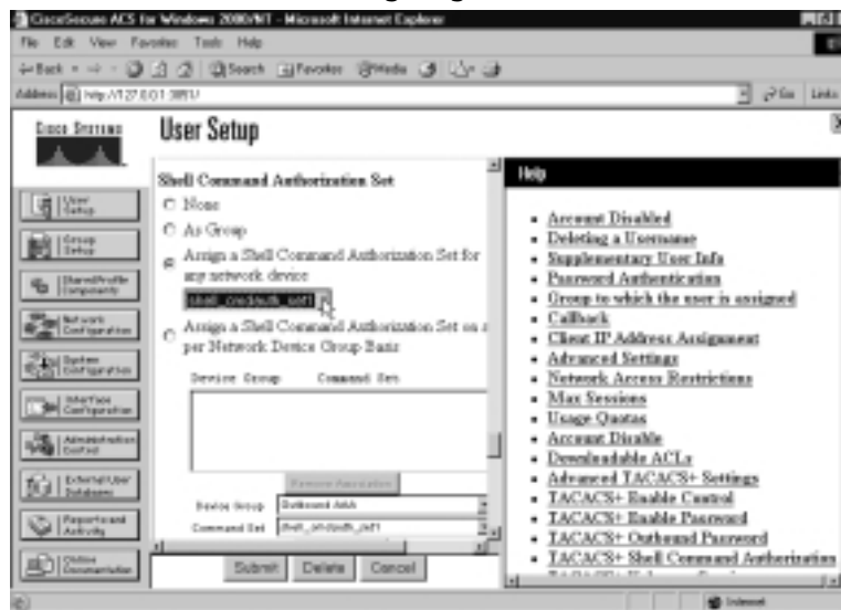
Figure 5.30 Cisco Secure ACS: Assigning Command Authorization Sets
